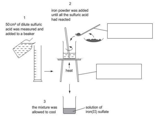
(a) Complete the boxes to identify the pieces of apparatus labelled. [2]
